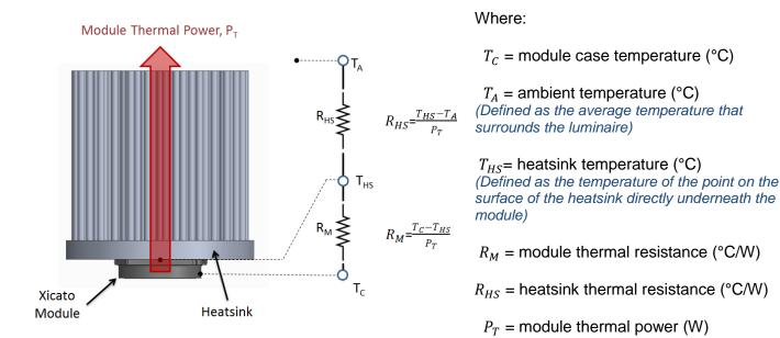
Furthermore, combining the module and heatsink thermal resistance equations give the following:
